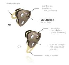
Quatron pulley system is specially designed for slacklining. Thanks to the "sheaveless" solution the dimensions of the whole system are minimized. The basic configuration of Quatron pulleys (9:1 base with 3:1 multiplier) creates a rigging system with the mechanical advantage of 27:1. MultiLock anchoring hole allows to anchor Quatron with 10 or 12 mm steel shackle that is always centered. Sealed ball bearings provide very high rigging efficiency even with higher
