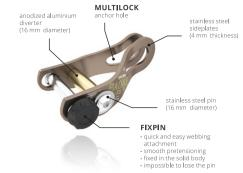
Paddle is an anchoring device for 50 mm wide webbing. It is designed to anchor tricklines up to 14 kN tension. Locking mechanism allows to pretension webbing in one way, whilst it is fixed in the other way. Paddle has smooth edges, so there is no danger of destroying the webbing. Thanks to middle axis with 26 mm diameter, the webbing retains more than 85% of its strength. Paddle FX can be attached to the anchor by most of available connectors (shackles, carabiners, quicklinks etc.).
